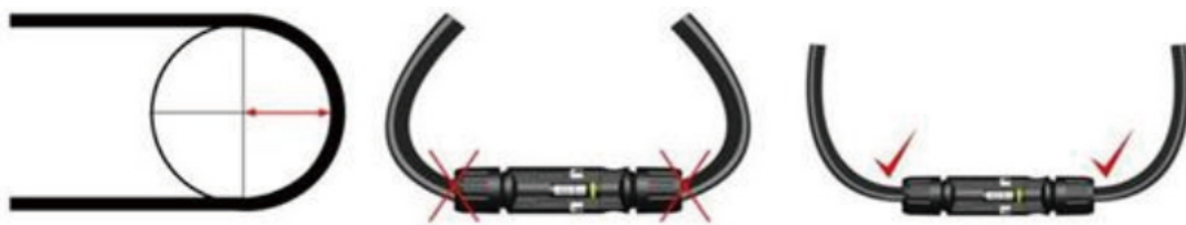
Figure 6-2 Minimum bending radius of the cable
